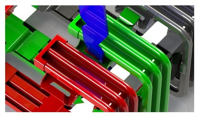
**Step 4** – While holding the red connector clip down with the blue separation tool use a flat head screw driver against the green link and push out the red link to separate the red connector from the green connector.
