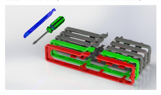
**Step 1** – Press the red and green links together so the lip of the red connector clip is clear of the green connector opening.
