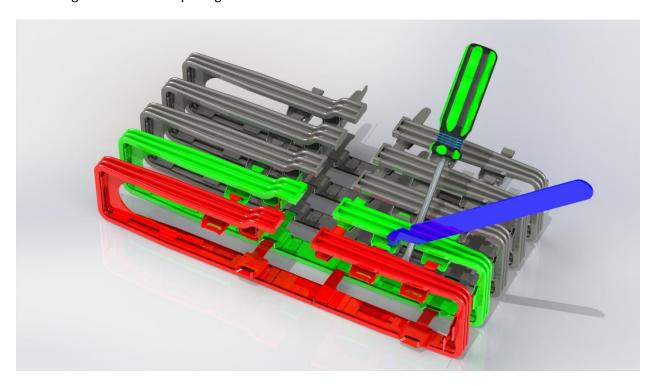
**Step 6** – While removing the blue separation tool from the green connector use the screw driver to make sure the links stay disassembled. Do the same process for the other four connectors.
