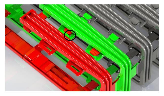
**Step 2** – Insert the point of the blue separation tool into the green connector opening next to the red connector clip.
