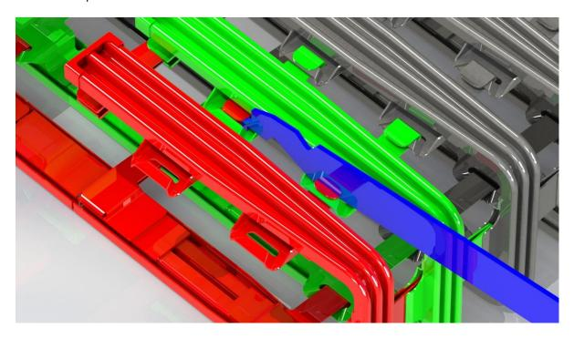
**Step 3** – Rotate the blue separation tool over the red connector clip while engaged in the opening of the green connector.
