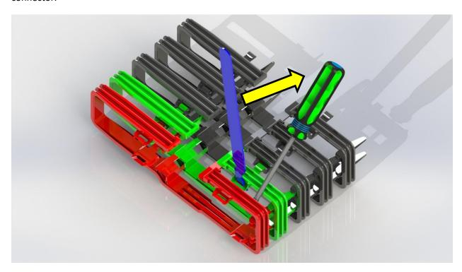
**Step 5** – Once the red connector clip is free of the green connector opening pull the blue separation tool from the green connector opening.
