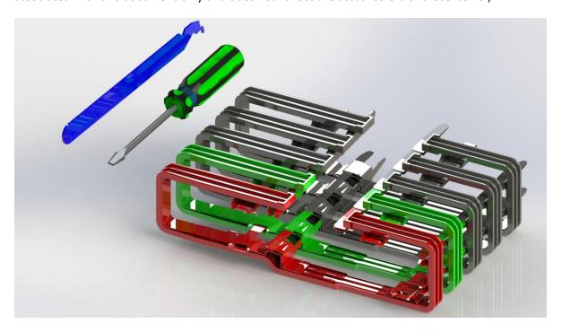
**Step 1** – Press the red and green links together so the lip of the red connector clip is clear of the green connector opening.
