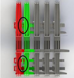
**View A** – The circle shows the location the blue separation tool will be inserted between the green connector opening and the red connector clip.
