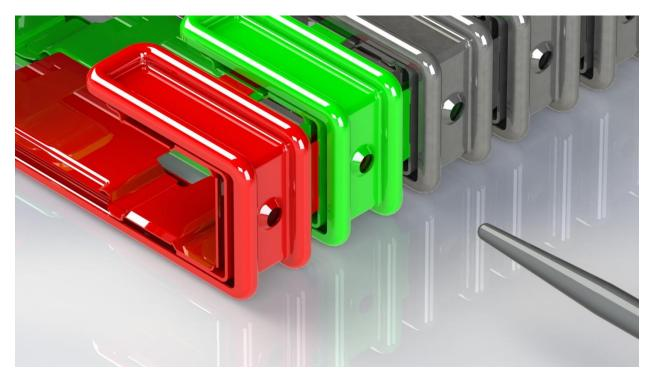
**Cut View** – This is an inside view of two links that have not been pressed together. Notice the connector does not clear the connector opening it is assembled in.
