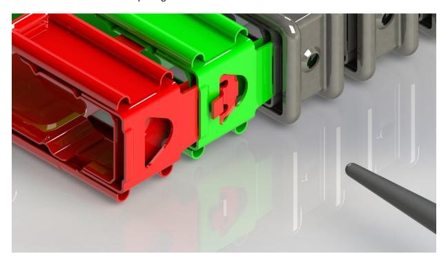
**Step 3** – Press the two links together to align the connector tip with the hole. Notice the connector clip clears the connector opening it is assembled in.
