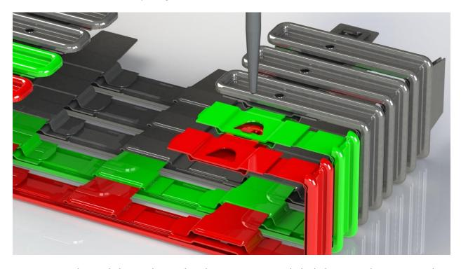
**Step 3** – Press the two links together to align the connector tip with the hole. Notice the connector clip clears the connector opening it is pushed in.
