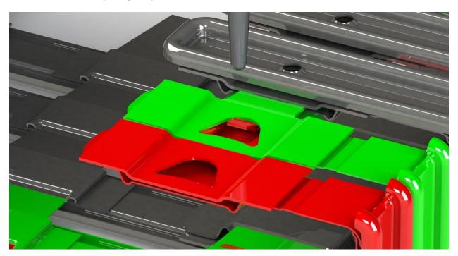
**Step 3** – Now that the links are pressed together insert the tool in the hole of the link you want to disassemble.
